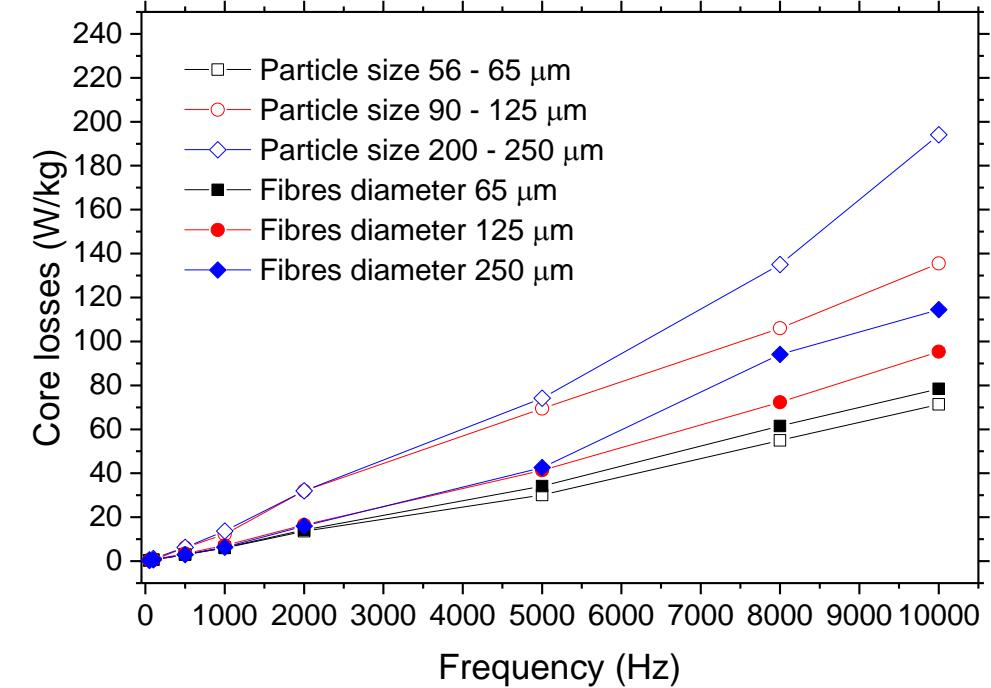
**FSMCs HAVE LOWER MAGNETIC LOSSES AS COMPARED TO SMCs**
